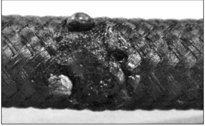
Photo 8 - Closeup of Power Steering Hose Failure of Steel Wire Braiding with Beading
