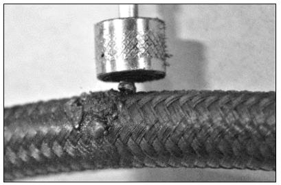
Photo 10 - Power Steering Hose Failure of Steel Wire Braiding with Beading and Magnet
