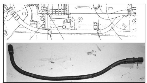
Photo/Schematic 9 - Power Steering Hose with Failure Location at Rear Support Clip
