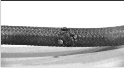
Photo 7 - Power Steering Hose Failure of Steel Ire Braiding with Beading
