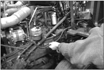
Photo 6 - Power Steering Hose Removed from Under and Inside Frame Rail – shown with Routing Displaced Upward and Outward
