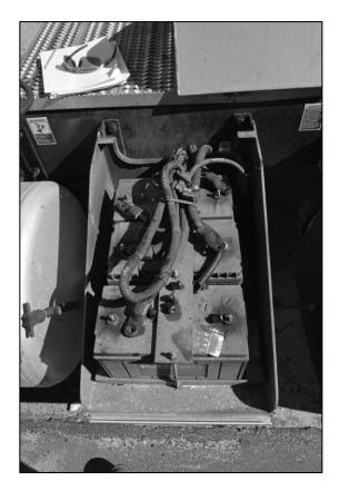
Photo 11 - Battery Box – mounted left side frame rail behind cab
